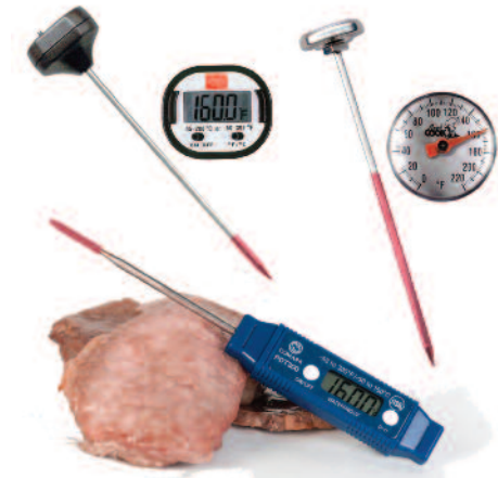
Figure 1. Dial instant-read thermometers (right) sense temperature in the bottom 2 inches of the stem. Digital instant-read thermometers (left and bottom) read temperature in the bottom 1/2-inch of the stem. A thin-tipped thermometer (bottom) can sense the temperature in thin meats.
