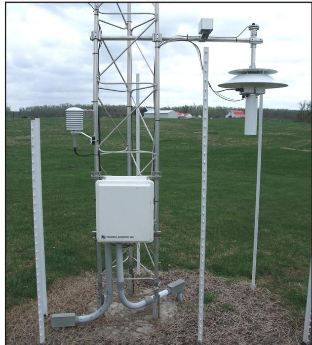
A KENTUCKY MESONET WEATHER STATION. THIS NETWORK OF AUTOMATED WEATHER AND CLIMATE MONITORING STATIONS WAS DEVELOPED BY WESTERN KENTUCKY UNIVERSITY.
